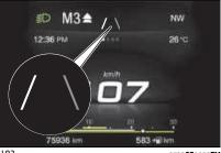
183 07226S0023EM When the system detects that the car has approached the lane line and is about to overtake it, the left line on the instrument panel display lights up yellow and red fig. 184.
