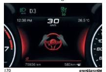
If the TJA system was deactivated because your hands were not on the steering wheel, the Active Cruise Control (ACC) will also be deactivated and must be reactivated
