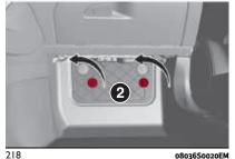
The number identifying the electrical component corresponding to each fuse is shown on the control unit cover.
