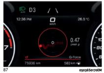
The displayed parameters are related to car stability, the graphs illustrate the trend of the longitudinal/lateral accelerations (G-meter information), considering gravity acceleration as a reference unit.
