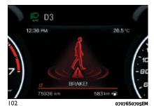
The acoustic and visual warnings before the system cuts in depend on the car speed. No acoustic/visual warning is generated at speeds slower than 20 mph (30 km/h). Acoustic/visual warning is generated at speeds faster than 20 mph (30 km/h), instead.
