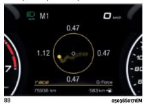
The displayed parameters are related to car stability, the graphs illustrate the trend of the longitudinal/lateral
