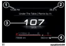
In RACE mode (where provided) the consumption indication index is not active and a sports gearshift indicator is displayed.
