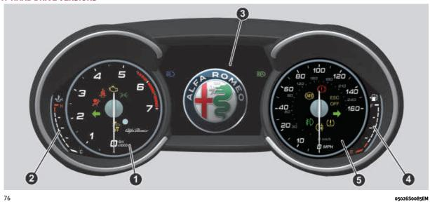
1. Rev counter 2. Digital engine oil temperature gauge with overheating warning light 3. TFT Display 4. Digital fuel level gauge (the triangle on the left side of the symbol indicates the side of the vehicle with the fuel filler) 5. Speedometer
