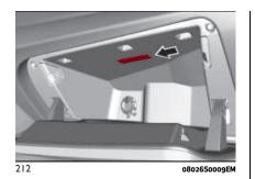
**Boot ceiling light**: act at the point indicated by the arrow fig. 213, remove the ceiling light and replace the lamp, making sure that it is correctly blocked between the contacts.
