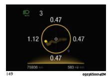
WARNING With braking system overheated, the Connect system communicates the condition. In this case, allow the system to cool for a few minutes by driving the car normally without operating the brakes.
