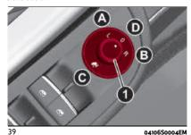
To adjust the selected mirror, use device (1) in the four directions.
