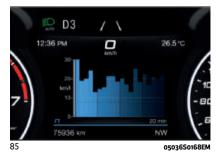
The screen graphically reproduces some parameters closely linked to the efficiency of the driving style, with a view to limiting consumption.
