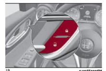
Pulling the handle, do not press the door lock/unlock button fig. 17 on the handle fig. 20.
