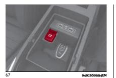
WARNING Do not connect devices with powers higher than 180W to the socket. Do not damage the socket by using unsuitable adaptors.
