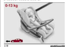
The child restraint system is restrained by the car seat belts, as shown in fig. 119 and it must restrain the child in turn with its own belts.
