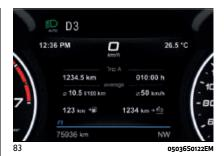
To reset the values, press and hold down the button on the right stalk fig. 84.
