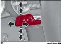
The main beam headlights are switched off by pushing the left stalk again. The instrument panel.
