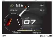
If the system intervention lasts longer than 10 seconds, an additional acoustic and visual warning will be provided by displaying a dedicated message on the instrument panel display to prompt the driver to regain control of the vehicle.
