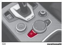
On the dashboard are the ON and OFF LED status. Moving the ignition device to MAR, the two LEDs switch on for a few seconds. If not, contact an Alfa Romeo Dealership. During the first seconds, the activation of the LEDs does not actually show the passenger protection status, but only checks its correct operation.
