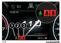
With the car travelling as speed lower than 12 mph (20 km/h), if a rear seat belt is unbuckled, the icon stays on with fixed light for a total of approximately 65 seconds.
