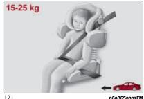
In this case, the child restraint system is used to position the child correctly with respect to the seat belts so that the diagonal belt section crosses the child's chest and not the neck, and the lower part is snug on the pelvis not the abdomen.
