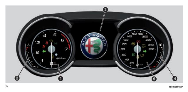
1. Rev counter 2. Digital engine oil temperature gauge with overheating warning light 3. TFT Display 4. Digital fuel level gauge (the triangle on the left side of the symbol indicates the side of the vehicle with the fuel filler) 5. Speedometer
