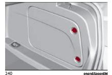
☐ remove the protective cover (1) fig. 241 and connect the positive cable terminal of the charger (usually red) to the positive terminal (+) of the battery;
