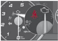
As soon as a speed threshold than 12 mph (20 km/h) (variable speed according to car conditions) is reached, with driver side seat belt or the passenger side seat belt (with occupant seated) unfastened, an acoustic signal is activated simultaneously with warning light & flashing for about 105 seconds. Once activated), this warning cycle stays active for the entire time if the car is moving faster 5 mph (8 km/h) or if reverse gear is not engaged or until the seat belts are fastened
